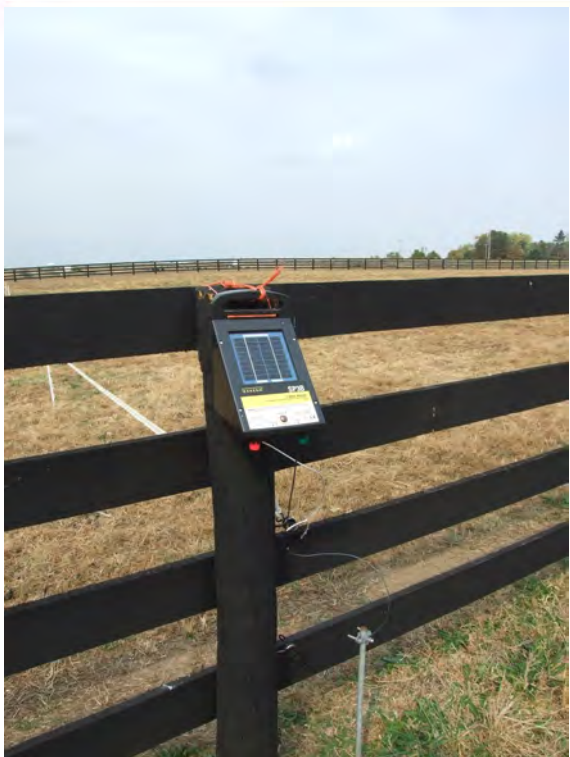
Many charger options are available: including those that need to be plugged into an electrical source, battery powered, or solar powered. Photo credit by Bob Coleman.
