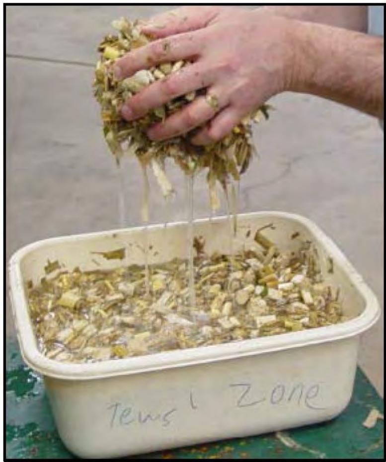
**Figure 3.** Skimming and removing the floating stover.
