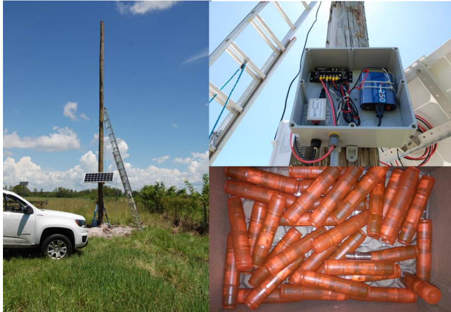
Figure 2: Final set-up of gateway tower on Big Cypress ranch fully operational on solar power (right upper panel), mounted on power pole specially erected by Heath Crum (Seminole Beef) and crew (left panel). Arrival of first batch of new LED red light sensors (right bottom panel)
