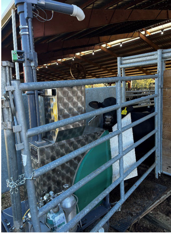
Figure 2. Measuring methane using the GreenFeed technology at the NFREC Feed Efficiency Facility at.
