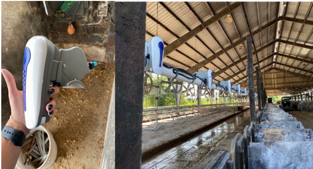
Figure 1. Representative images of the individual unit of the SmartSoaker (A) and the system installed (B) in the barn where animals were housed for the period of the study ( \pm 45d ).
