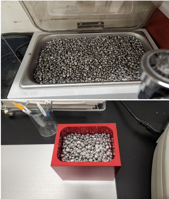
Figure 1. Examples of use of metal beads in a water bath (top) or plastic carrier on a heating plate (bottom).
