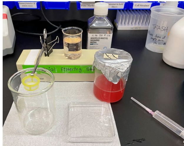
Figure 11. Illustration of setup for filtering medium containing oocytes. Shown are a 10 mL syringe fitted with an 18 g needle and smaller beaker containing oocyte washing medium after collection of oocytes (ready for filtering). The binder clip is attached to the hemostat to hold the filter at the same level as the empty beaker.
