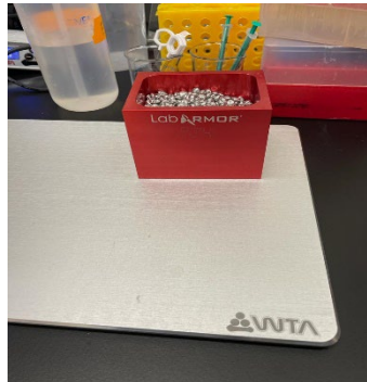
Figure 1. Small bead blocks with metal beads. Use of beads eliminates the algal contamination often seen with water baths.
